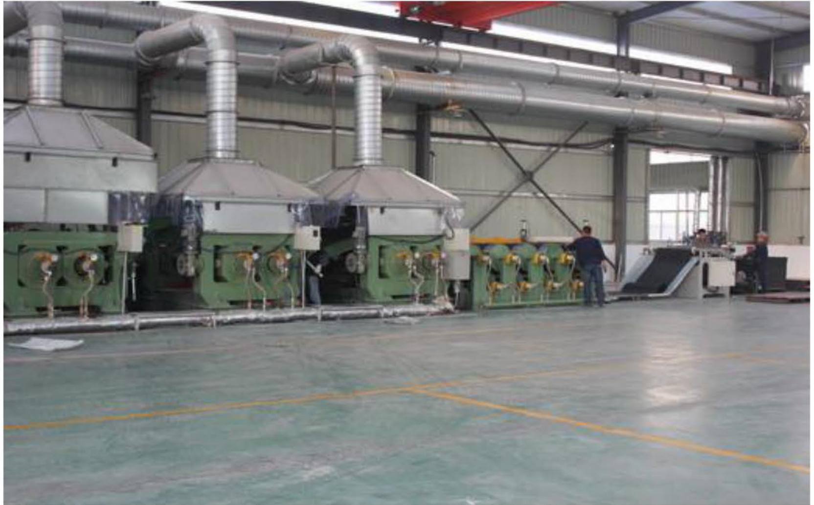
Middle & Balance PVC layer production line
